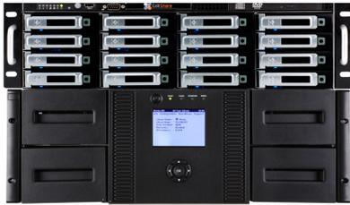
Ark Disk server and 48-slot LTO-6 tape library, for a combination of nearline disk-based and energy-saving tape-based archiving
